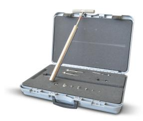
Used to determine the relationships between moisture content, density, and penetration resistance. These relationships are used with a previously prepared family of moisture-penetration curves as a rapid field test to determine the approximate amount of moisture in the soil
