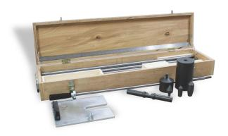
Used to assess the thickness of various layers (strata) during compaction testing and to gauge the relative density of both engineered fills and naturally occurring loose soils.
