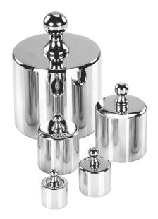
• These weight measurements play a crucial role in conducting regular and periodic checks of the balances. By utilizing these weights, the process of balance verification and validation is not only facilitated but also enhanced. These weight values serve as fundamental reference points against which the existing balances are compared during routine examinations.
