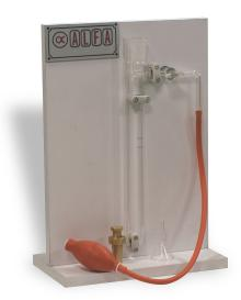
Used to determine the fineness of hydraulic cement, using the Blaine air-permeability apparatus, in terms
