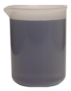
A plastic beaker in engineering testing laboratories is used for holding, mixing, and heating liquids or chemicals. It is lightweight, durable, and resistant to breaking, making it ideal for everyday use in various laboratory procedures where glass beakers may be too fragile or impractical.
