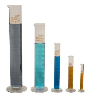
A glass measuring cylinder in engineering testing laboratories is used for accurately measuring the volume of liquids or small amounts of substances. Its clear markings and wide cylindrical shape ensure precise volume measurements during experiments, chemical analysis, or sample preparation.
