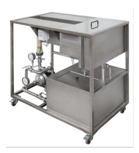
• The unit is self-contained service module providing a controlled flow of water to a range of optional accessories.
